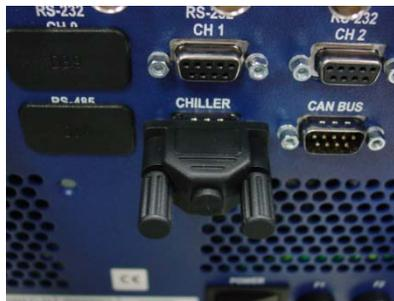
Figure 2-12 Chiller Interlock Connector
