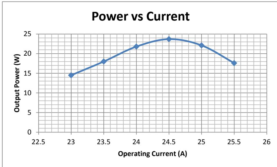
Figure 3-2 Example of Laser Performance Dependence on the Operating Current
