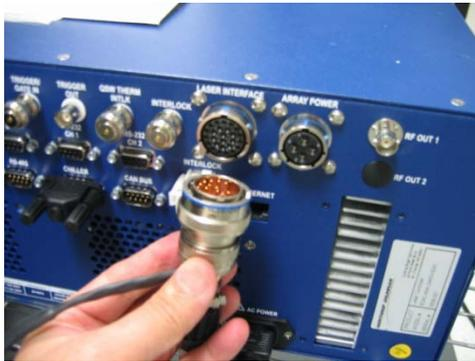
Figure 2-10 Diode Power Cable
