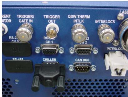
Figure 2-14 BNC Interlock Connection
