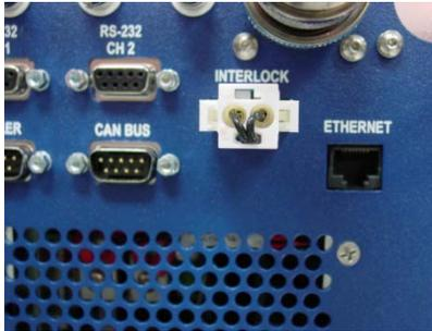
Figure 2-13 White Interlock Connectors
