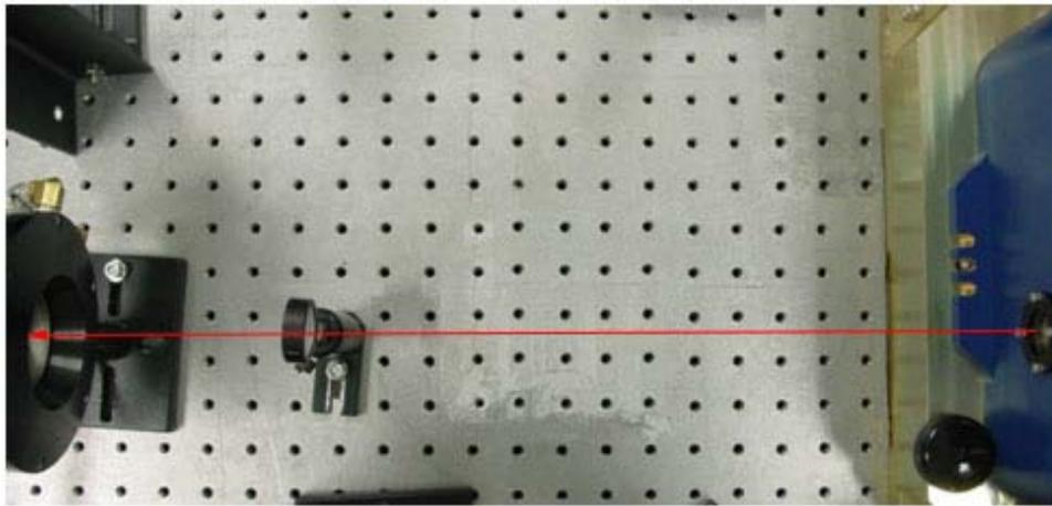
Figure 2-1 Basic Setup for the Laser Power Test
