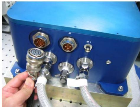
Figure 2-6 Signal Connection
