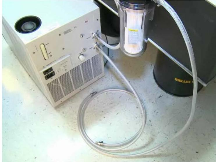
Figure 2-3 Chiller Assembled with Coolant Hoses and Filter
