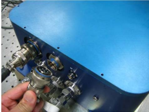
Figure 2-7 Diode Power Connection
