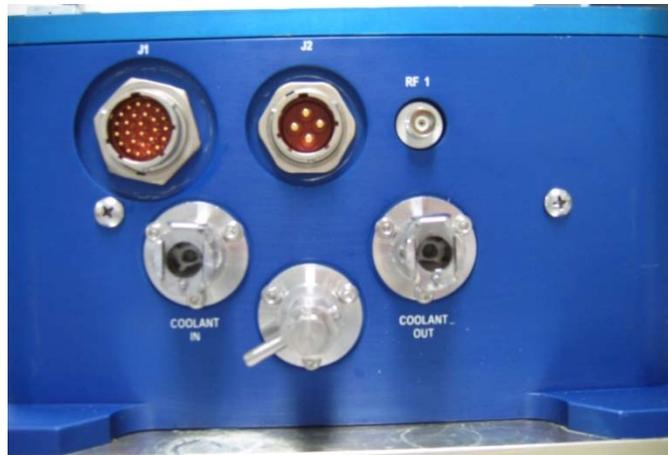
Figure 2-4 Connectors on the rear panel of the Patara-IR TEM<sub>00</sub> laser
