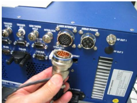
Figure 2-9 Laser Signal Cable
